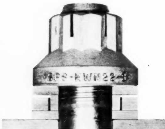
Before Preloading. Inner PLI ring has not been compressed. Outer PLI ring can be rotated freely by wire in feeler hole. Nut is then tightened until outer ring cannot be rotated.
